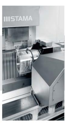
Each work place has one milling and one turning spindle, enabling precise and powerful 5-axis complete machining. Sides 1–5 are milled and turned in the first workstation, at the same time sides 2–6 of the same workpiece in the second.
