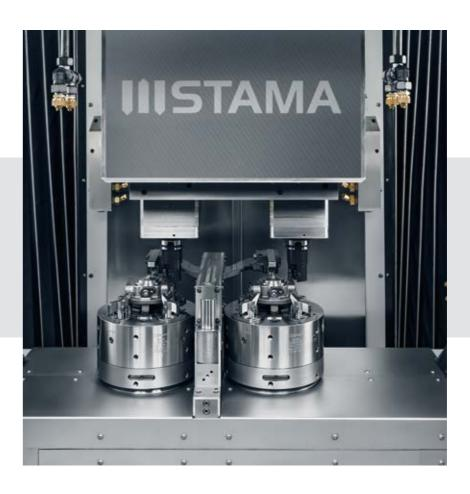
Loading, unloading and setting up parallel to main time on two place milling-turning centers reduces non-productive time and ensures more efficient quality assurance, lower logistics expenses and more personal responsibility for the operator.
