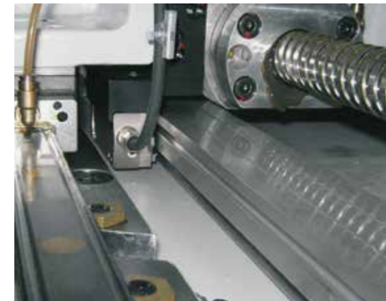
Highest precision: glass scales, digital drive technology and absolute path measurement systems allow high acceleration with equally high contour accuracy.
