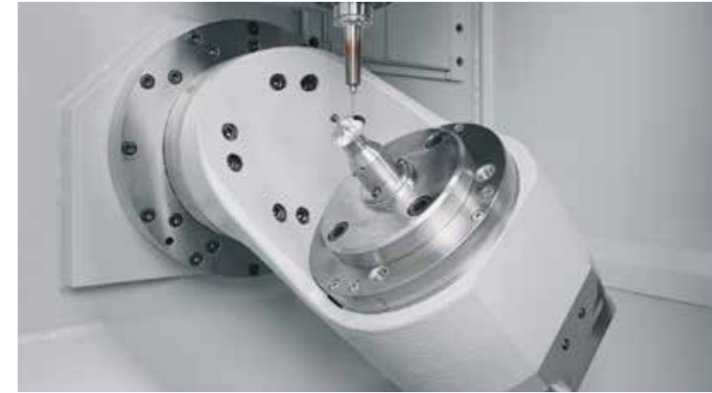
FZ 08 S five axis: Integrated 2-axis rotary table (BC kinematics), maintenance-free torque drive technology and automatic tool change with the pick-up method.
