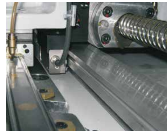
Highest precision: Glass scales and digital drive technology allow high acceleration with equally high contour accuracy.
