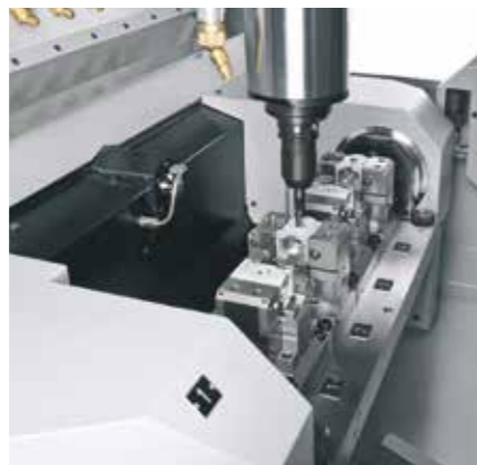
FZ 12 W: Machining center with automatic tool change using the pick-up method and tool changing device for loading and unloading during machining.
