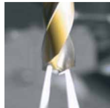
Internal cooling via the spindle up to 70 bar; also available with a frequencycontrolled pump
