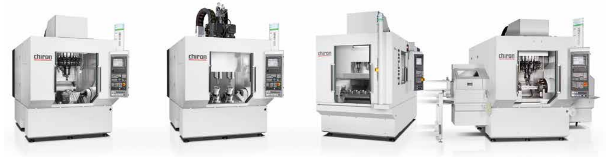
FZ 15 S five axis: Fast precision machining center with a basket tool changer and a 2-axis swivel rotary table for 5-axis simultaneous and complete machining. Workpieces can be machined with high surface quality in one set-up.
