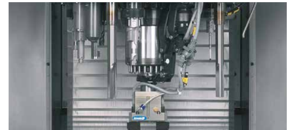
Workpiece gripper in the main spindle for machine-integrated workpiece handling
