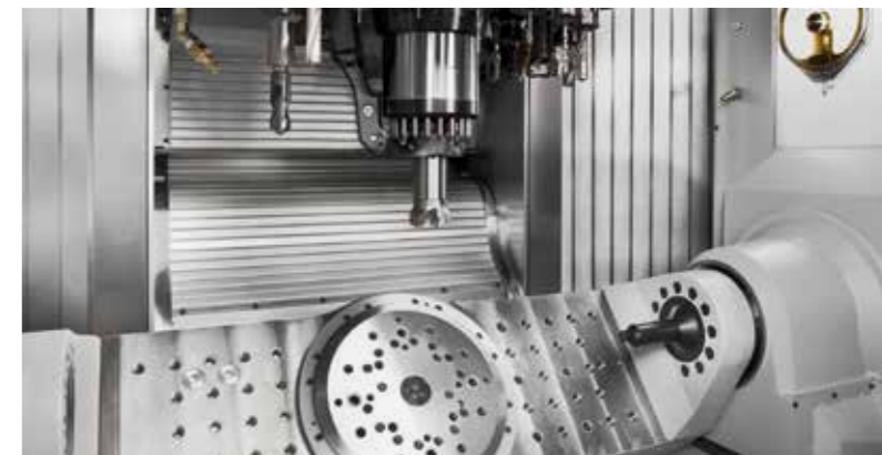
FZ 15 S five axis: Fast precision machining center with the fast CHIRON basket tool changer and a 2-axis swivel rotary table. High productivity, with chip-to-chip times as short as 1.7 seconds and tool changing times from 0.9 seconds.
