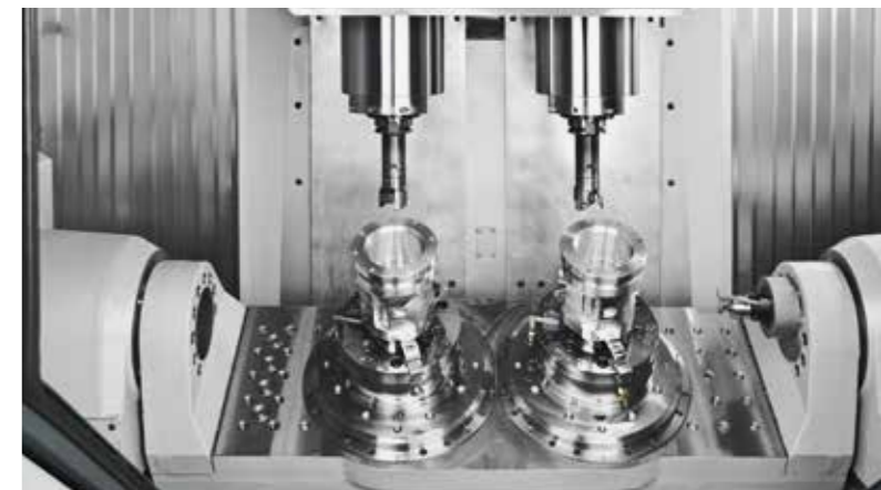
DZ 15 S five axis: Doubled productivity with minimal space requirements: fast double-spindle machining center with a 2-axis swivel rotary table with two face plates for efficient complete machining with five simultaneously controlled axes.
