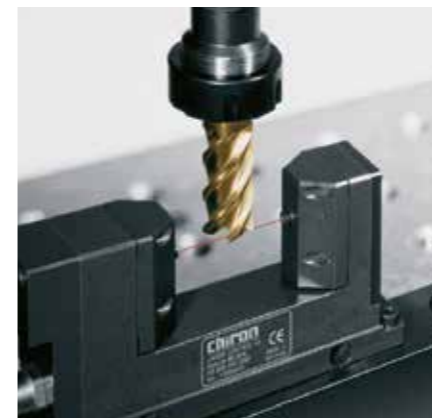
CHIRON laser control for tool breakage checks, for tool measurement and for machine compensation.
