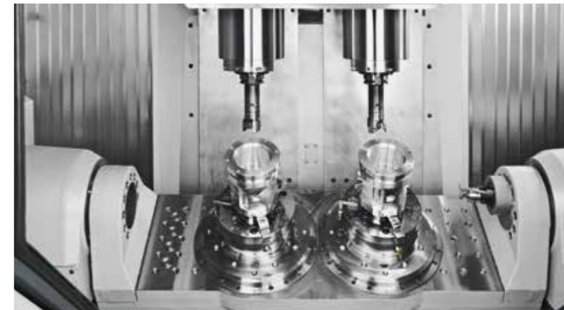
DZ 18 S five axis: Doubled productivity with minimal space requirements: fast double-spindle machining center with a 2-axis swivel rotary table with two face plates for efficient complete machining with five simultaneously controlled axes
