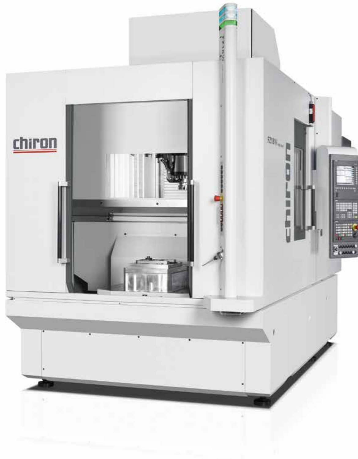
FZ 18 W Machining center with basket tool changer (20 tool places) and workpiece changing device 0°/180°, enabling loading and unloading during machining.
