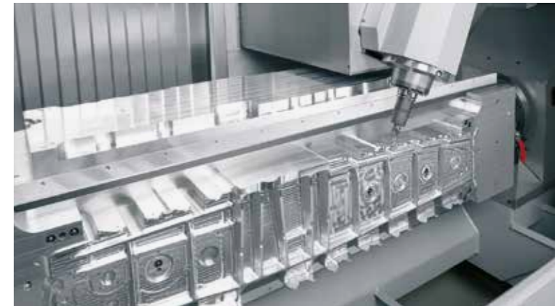
MILL 2000: Combination of a NC swivel head and a standard rotary table basic device. The swivel plate can be customized according to our customers' requirements; for instance 4-sided due to a clamping cube.
