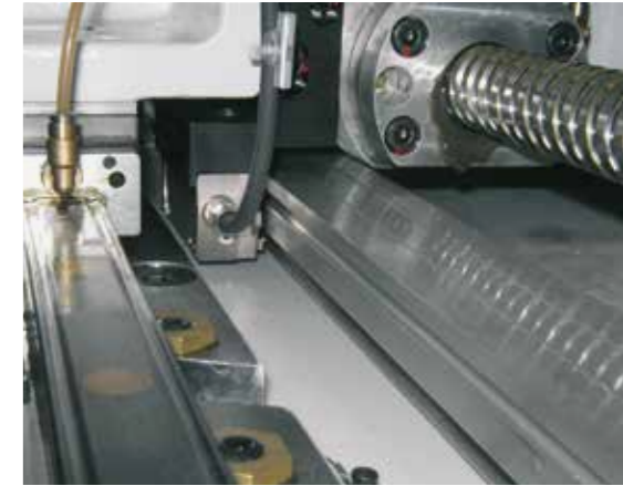
Highest precision: Glass scales and digital drive technology allow high accelerations with the same contour accuracy. Machines with traverse paths of more than 4,500 mm in X are equipped with linear motors.
