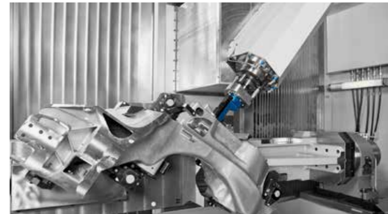
MILL 3000: Combination of a NC swivel head and the basic device. Achieve maximum productivity using the High Dynamics package.
