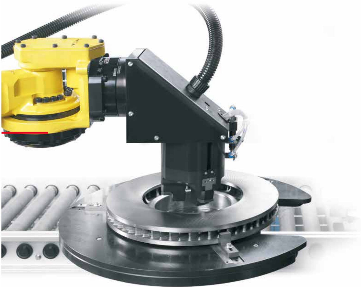
Space-saving integration of an articulated arm robot for removing finished parts.
