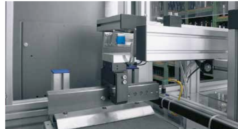
Space-saving integration of an articulated arm robot for removing finished parts.
