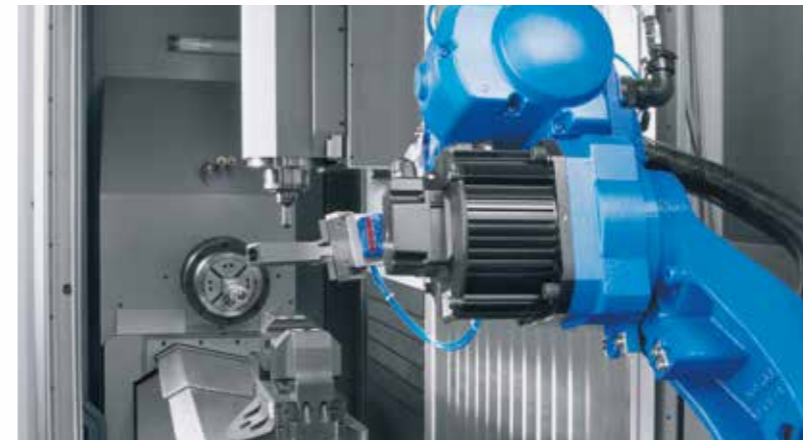
Space-saving integration of an articulated arm robot for removing finished parts.
